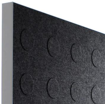
The screens consists of a sound-absorbent acoustic filling mounted on an aluminium frame. Both sides of the screen are upholstered in compressed sound-absorbent polyester felt.
